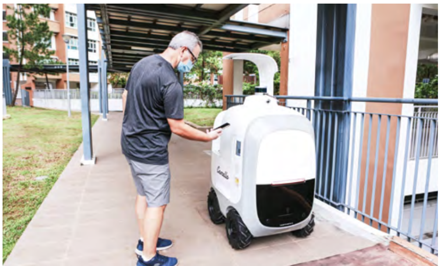
Camello, a last-mile delivery robot, was developed by OTSAW to disrupt and transform the current logistical process. It has a 100-litre compartment volume which can carry up to 20 kg and is also equipped with UV-C LED to prevent cross-contamination between different users.
