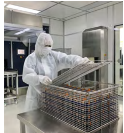
Clean manufacturing is necessary in the production of components for the power electronics, energy management and thermal management systems for electrical vehicles. Image: LPW Reinigungssysteme.
