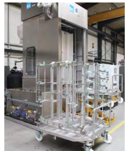
For cleaning, using the turntable system, car body parts, up to 2,200 mm long, e.g. extruded profiles, are fixed vertically and positioned precisely. Image: BvL Oberflächentechnik.
